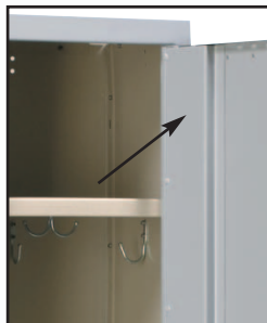
Marquis Student Lockers include a 3" wide 18 gauge full height door stiffener spot welded to the inner door face and MIG welded to the hinge side as well as to the top and bottom door flanges providing a rigid torque-free door. A 1-1/2" wide stiffener will be furnished for 9" wide Marquis doors.
