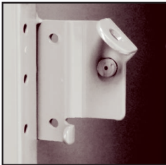
11 gauge single-point latch with pry resistant lug is MIG welded to Hollow-T frame
