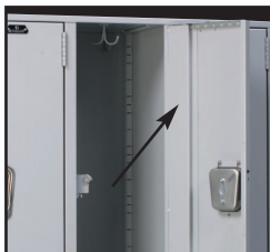
Marquis Protector lockers include a 3" wide 18 gauge full height door stiffener spot welded to the inner door face and MIG welded to the hinge side as well as to the top and bottom door flanges providing a rigid torque-free door. A 1-1/2" wide stiffener will be furnished for 9" wide Marquis doors.
