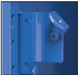
11 gauge single-point latch with pry resistant lug is MIG welded to Hollow-T frame
