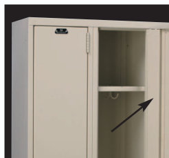
Marquis Booksafe III lockers include a 3" wide 18 gauge full height door stiffener spot welded to the inner door face and MIG welded to the hinge side as well as to the top and bottom door flanges providing a rigid torque-free door. A 1-1/2" wide stiffener will be furnished for 9" wide Marquis doors.
