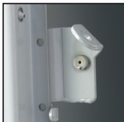
11 gauge single-point latch with pry resistant lug is MIG welded to frame
