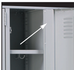
Upgrade to Premier Series Graduated lockers which include a 3" wide 18 gauge full height door stiffener spot welded to the inner door face and MIG welded to the hinge side as well as to the top and bottom door flanges providing a rigid torque-free door. A 1-1/2" wide stiffener will be furnished for 9" wide Premier Series doors.
