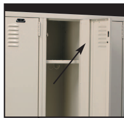
Upgrade to Premier Series Classmate lockers which include a 3" wide 18 gauge full height door stiffener spot welded to the inner door face and MIG welded to the hinge side as well as to the top and bottom door flanges providing a rigid torque-free door. A 1-1/2" wide stiffener will be furnished for 9" wide Premier doors.
